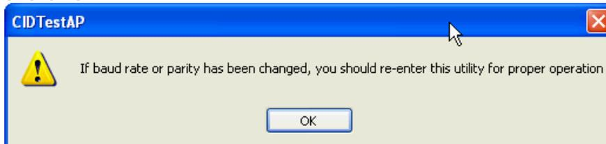
Note: This message is displayed every time you choose the Configure command. If you have just changed the baud rate or the parity (for RS232 interface), the Configure command will fail and display an error message. In that case, you need to exit the utility and re-start it with the new baud rate or parity.
