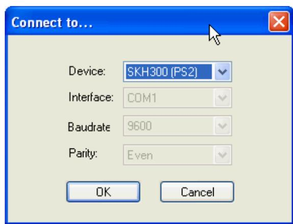
**TIP:** If your iButton reader is in serial mode and you access the reader in PS/2 mode, you can still check the firmware version and the configuration of the reader. This is useful if you can not
